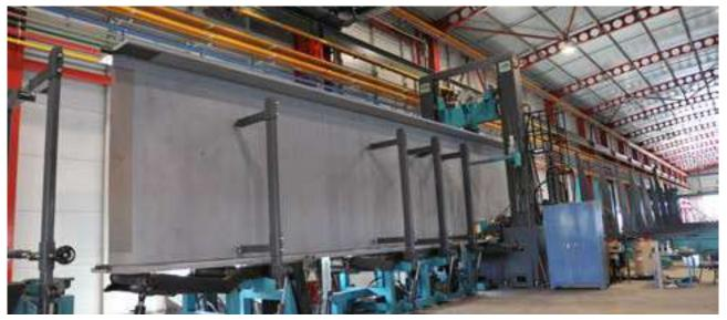
All weldings were made on the basis of approved WPS. WPSs were made in accordance with EN ISO 15609-1: 2004. WPS reported on the WPQR certified welding method. During the welding phase, it was possible to modify it under the supervision of the welding co-ordinator.
