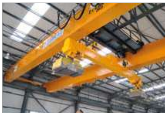
Double girder cranes 2x8t x 29m (Sidma S.A.)
